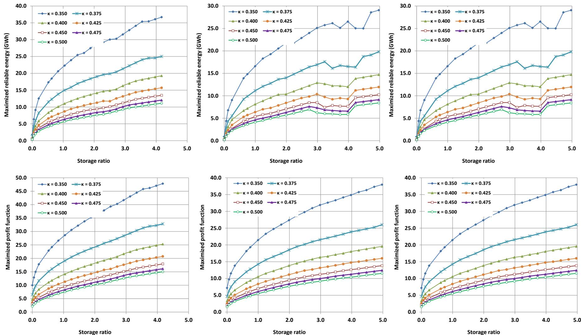
*Plots of maximized energy for monthly reliability level 99% (upper panels) and maximized profit (lower panels) as function of storage ratio (storage capacity/mean annual inflow) and the shape parameter, for capacity factor CF = 80% (from left to right: Achelous, Evinos, and Boeotikos Kephisos inflow data)*
