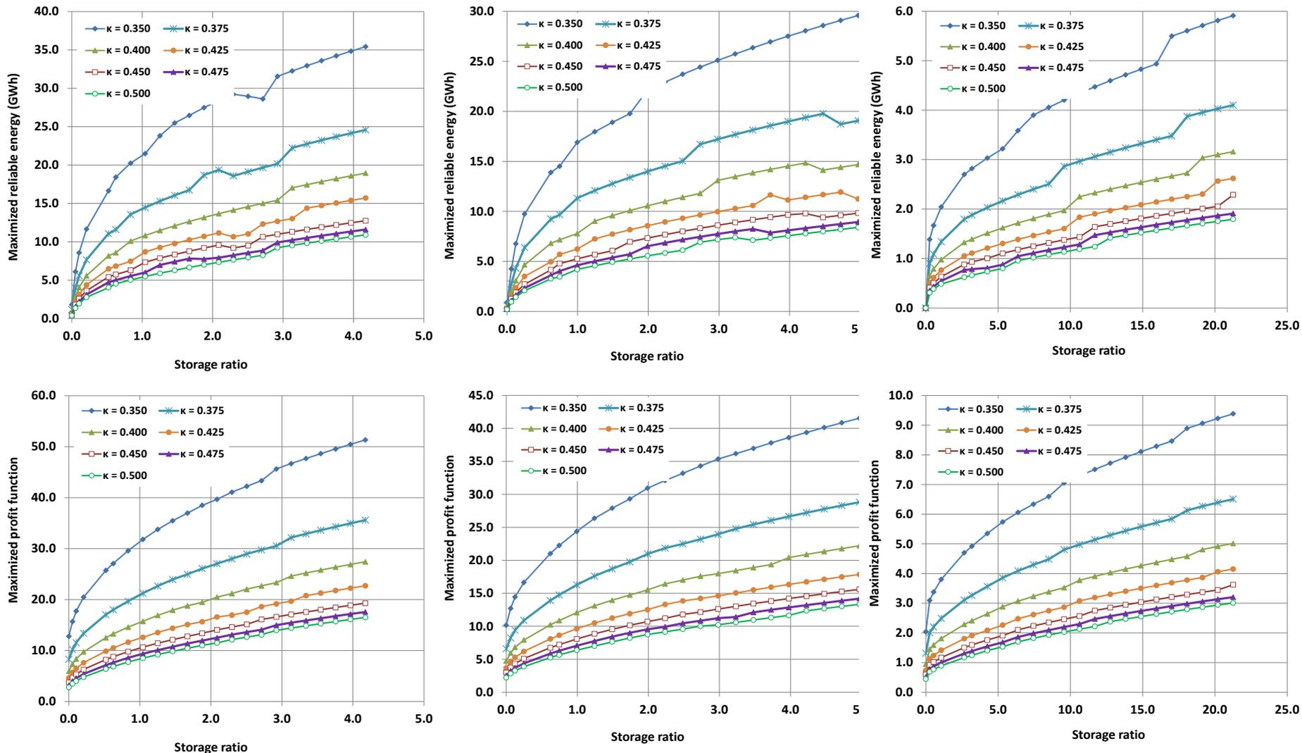
*Plots of maximized energy for monthly reliability level 99% (upper panels) and maximized profit (lower panels) as function of storage ratio (storage capacity/mean annual inflow) and the shape parameter, for capacity factor CF = 20% (from left to right: Achelous, Evinos, and Boeotikos Kephisos inflow data)*
