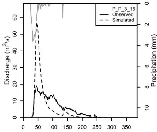
**Figure 7.1: Observed and simulated flood events at the Pievepelago hydrometric station.**
