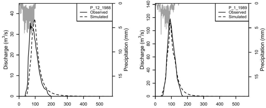
**Figure 7.9: Observed and simulated flood events at the Panagia bridge (Peristerona) hydrometric station.**
