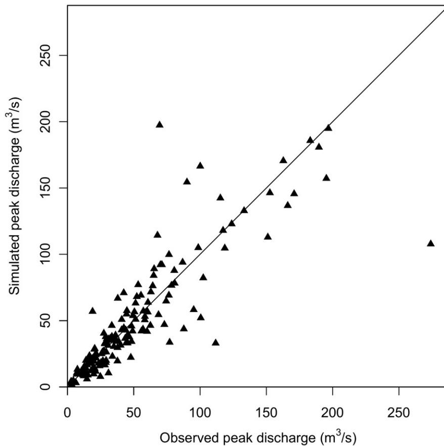
**Figure 5.1: The observed and simulated peaks for the 160 flood events.**
