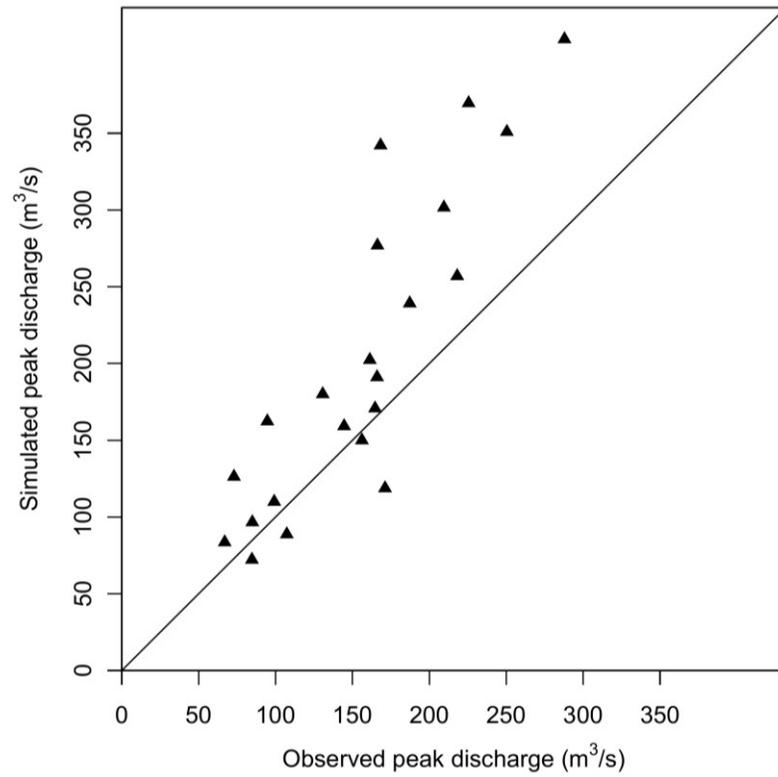
**Figure 5.6: The observed and simulated peaks for the Vetto flood events.**
