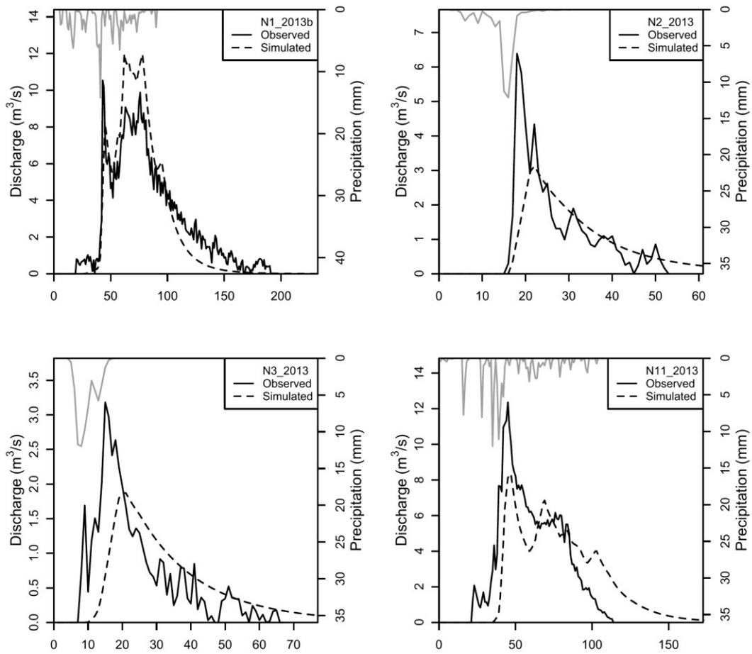
**Figure 7.8: Observed and simulated flood events at the Kalamata (Nedontas) hydrometric station.**
