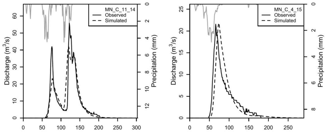
**Figure 7.6: Observed and simulated flood events at the Castrocaro hydrometric station.**
