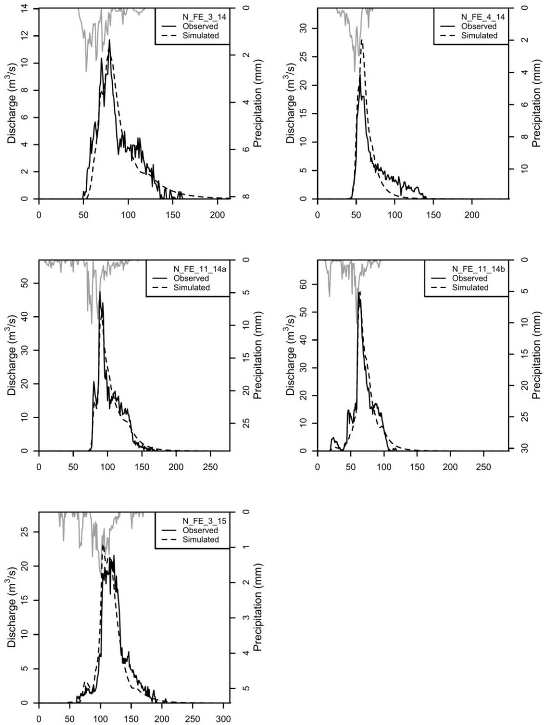
**Figure 5.5: Observed and simulated flood events at the Ferriere hydrometric station.**
