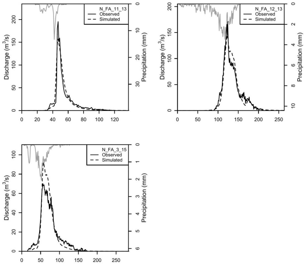
**Figure 7.5: Observed and simulated flood events at the Farini hydrometric station.**
