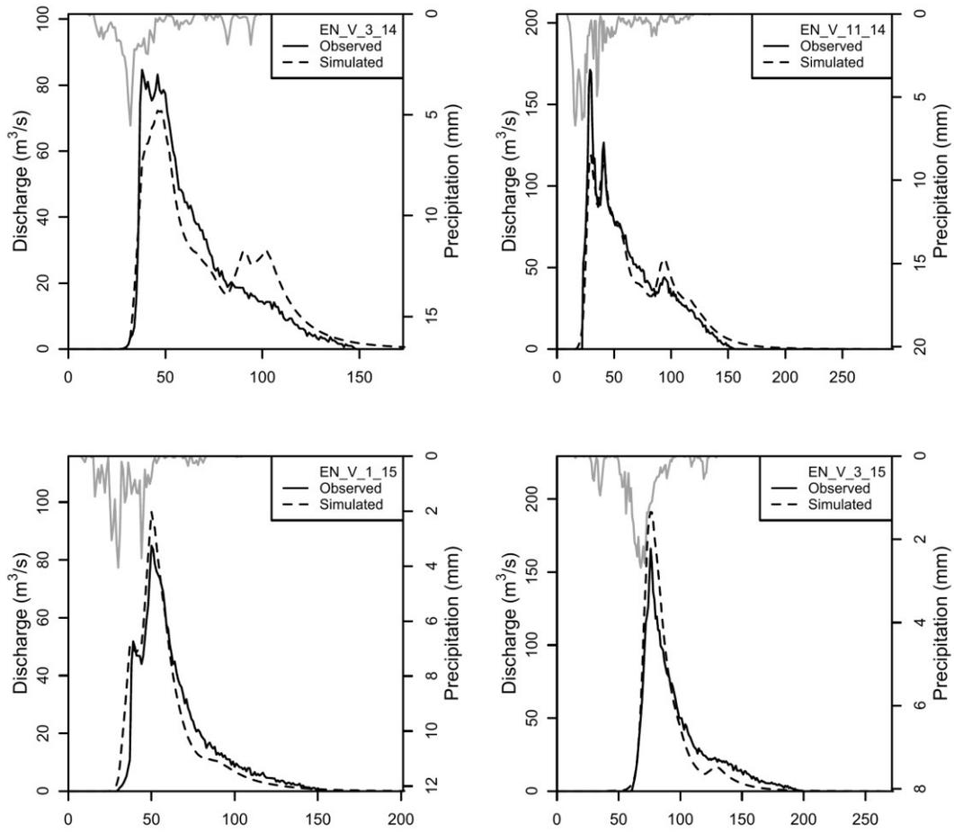
**Figure 5.7: Observed and simulated flood events at the Vetto hydrometric station.**
