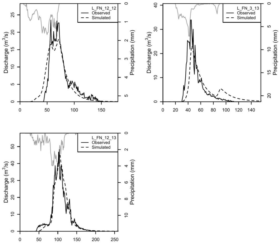
**Figure 7.4: Observed and simulated flood events at the Fanano hydrometric station.**
