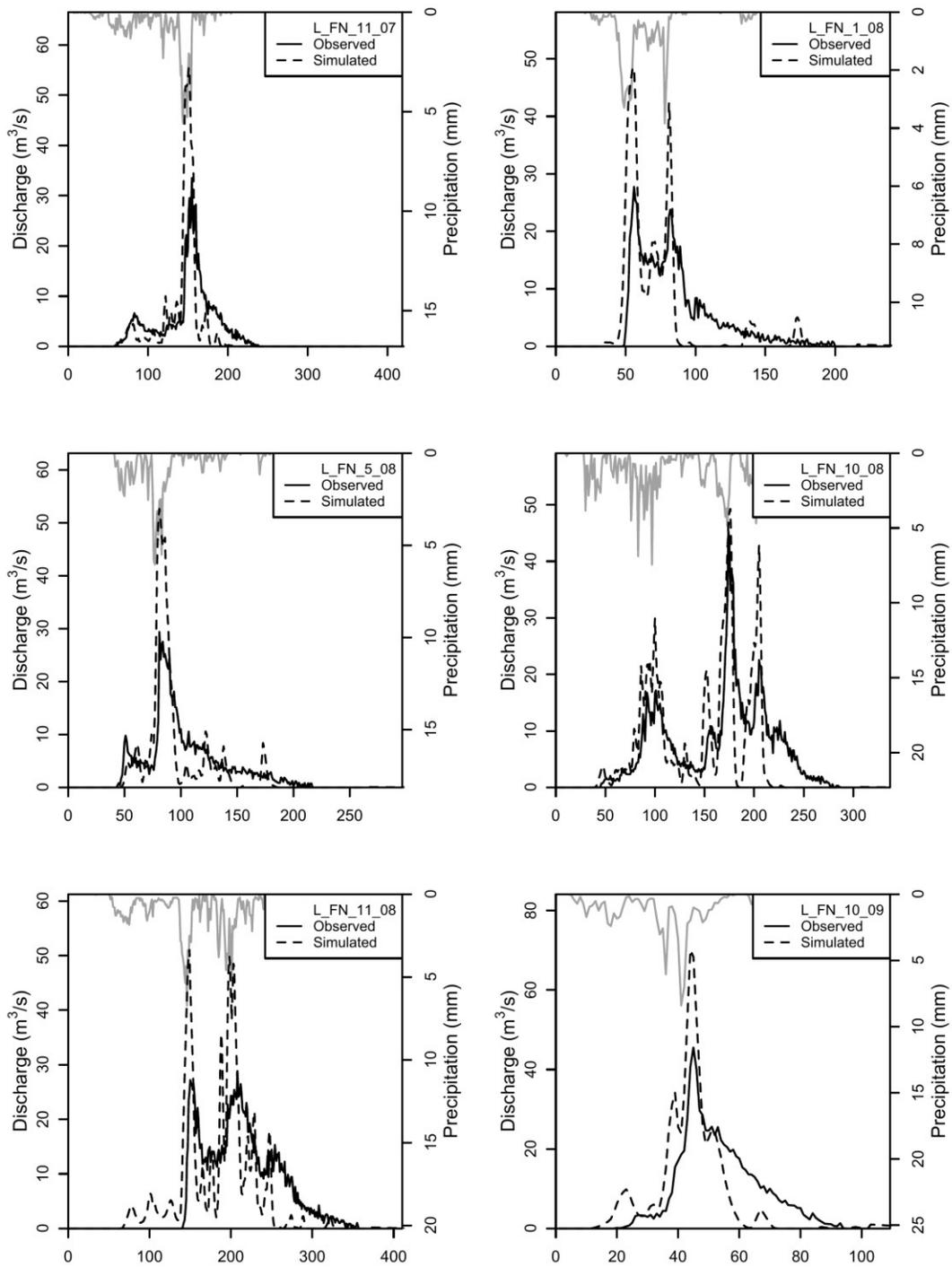
**Figure 5.8: Characteristic examples of observed and simulated hydrographs from Fanano using the triangular SUH.**
