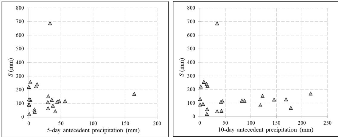
**Figure 5.11: The maximum potential retention,  $S$ , as a function of the 5- (top) and 10-day (bottom) antecedent precipitation for the Vetto catchment.**
