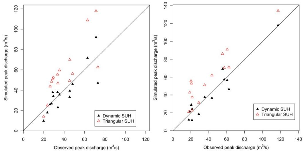
**Figure 5.9: Observed and simulated peak discharges using the dynamic SUH and the triangular SUH for Fanano (left) and Peristerona (right).**
