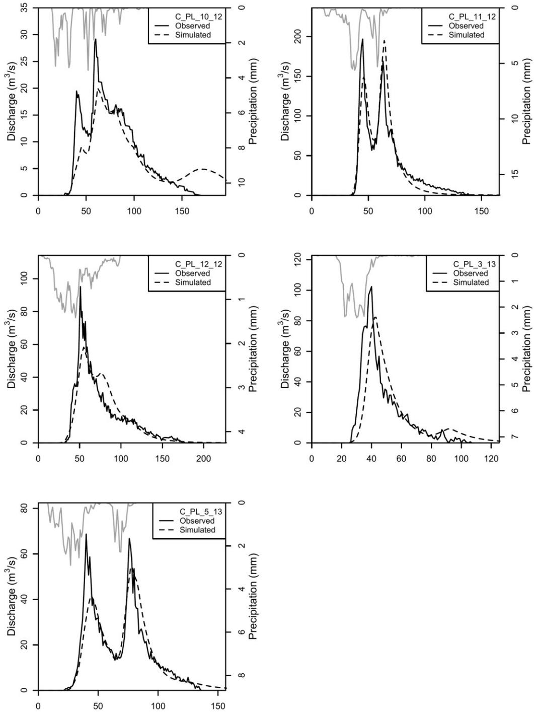
**Figure 7.3: Observed and simulated flood events at the Ponte Lamberti hydrometric station.**
