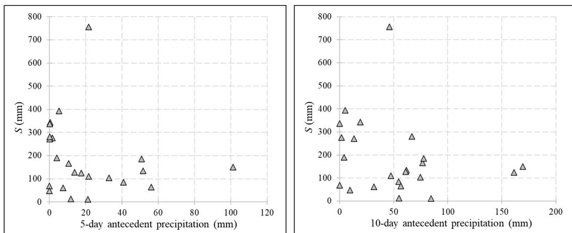
**Figure 5.10: The maximum potential retention,  $S$ , as a function of the 5- (top) and 10-day (bottom) antecedent precipitation for the Ferriere catchment.**
