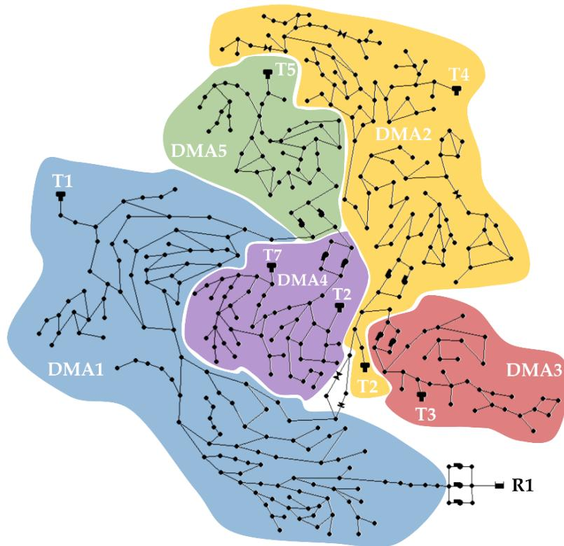
**Figure 1.** Visualization of the C-town WDN with five DMAs highlighted.
