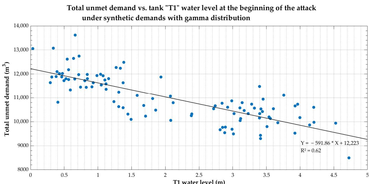
**Figure 3.** Relationship between the water level in tank “T1” when the cyber-physical attack starts and the resulting total unmet demand, simulated using synthetic hourly demand patterns with a gamma distribution.
