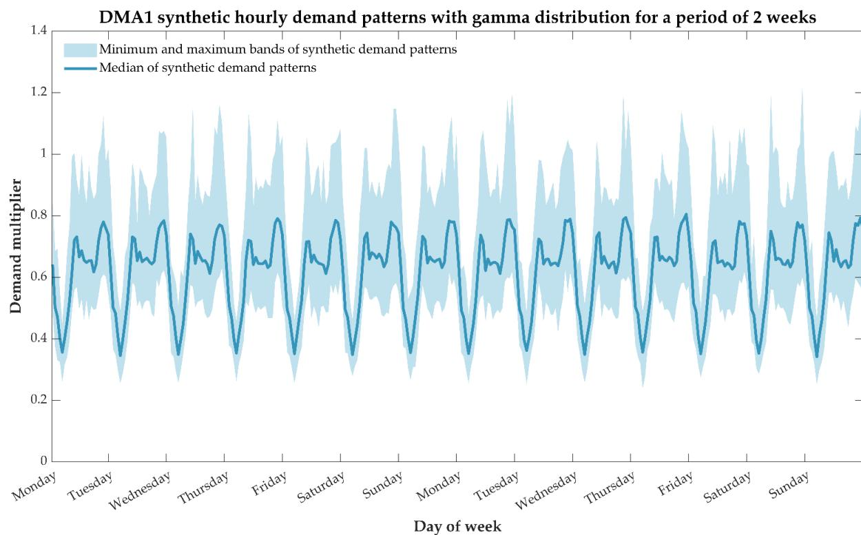
**Figure 2.** Median and outer bands (minimum and maximum) of the synthetic hourly demand pattern timeseries with gamma distribution generated for DMA1.
