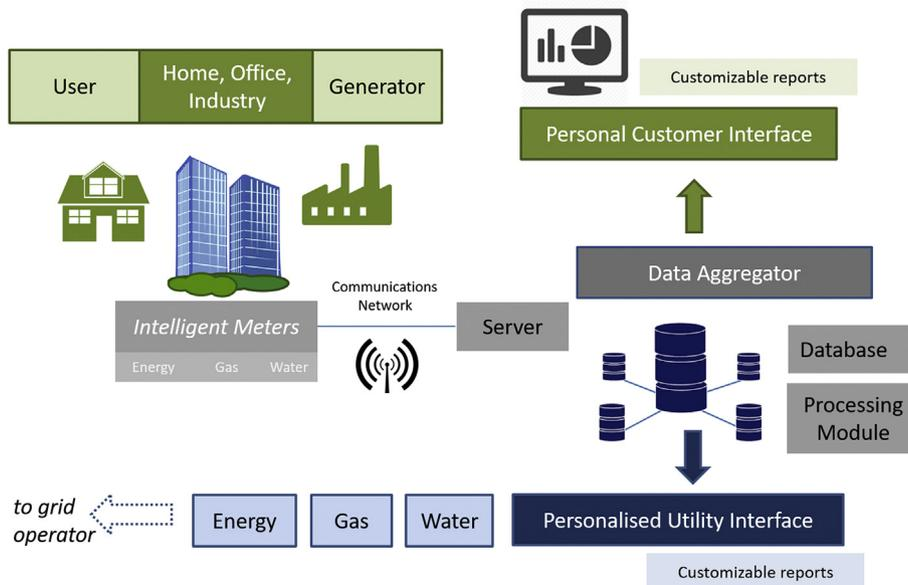
Fig. 1. Digital multi-utility system architecture overview.
