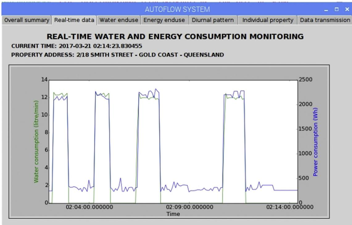
Fig. 2. Concurrent water-electricity demand signal (5s; L/min and Wh) (Autoflow screen shot).
