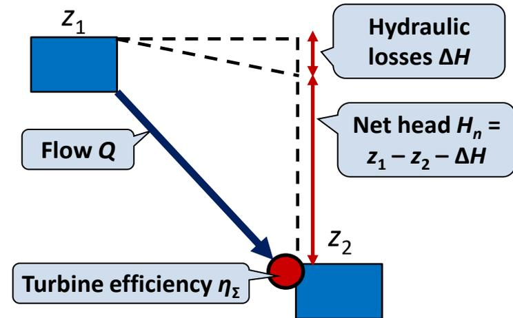
**Power production:  $P = \eta_z \gamma Q (\Delta z - \Delta H)$**
