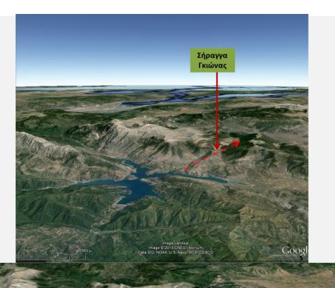
The largest SHPP across Mornos aqueduct is Giona, which operates since 1987. It is located near the city of Amfissa, belongs to the PPC and exploits a part of the water volume transported to the city of Athens. The operational discharge fluctuates from 7.8 to 14.5 m<sup>3</sup>/s, and the head from 30.0 to 66.1 m. The installed power is 8.67 MW and the mean annual electrical energy production is about 34 GWh.
