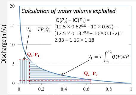
Probability of exceedance For one-year operation,  $T = 31.56 \times 10^6$  s  $V_0 = 31.56 \times 0.132 \times 5 = 20.8 \text{ hm}^3$
