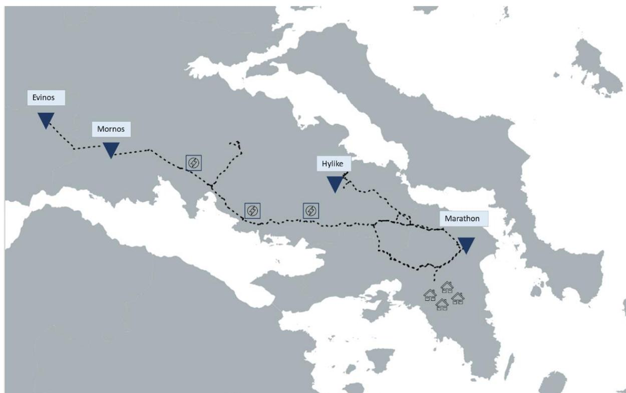
**Figure 6.2.** Configuration of Athens' water supply system.
