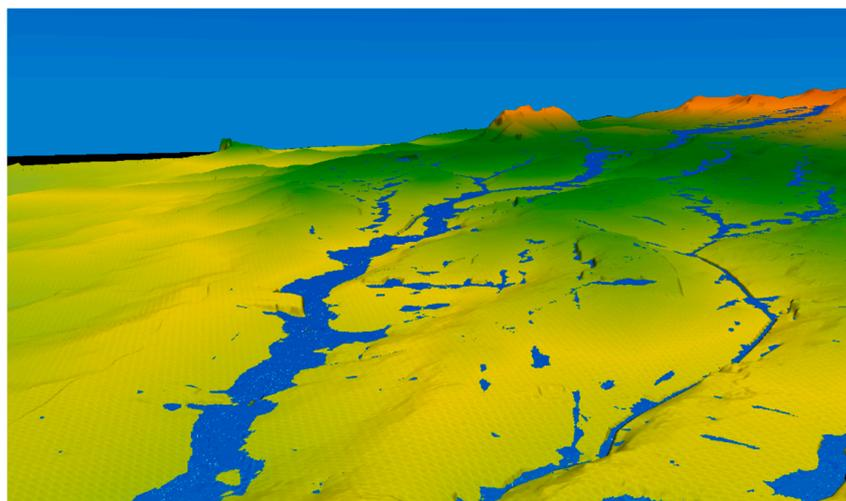
**Figure 9.** Example of a 3D view of the simulated flood scenario based on the HEC-RAS 6.3 software.
