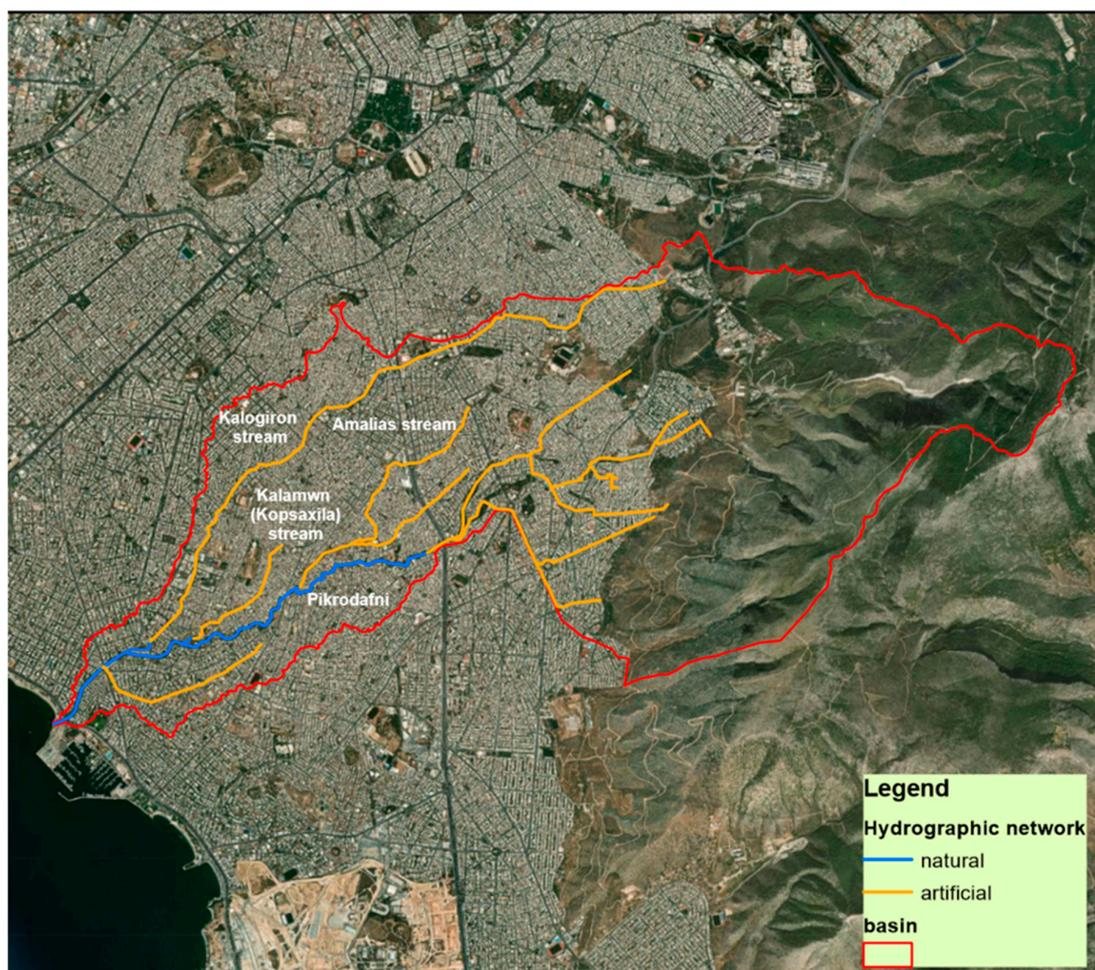
Figure 5. Hydrological network of Pikrodafni’s river basin, including reaches with a natural riverbed and ones with technical works.
