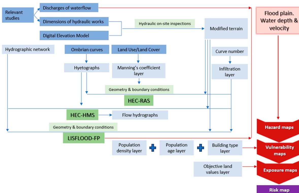
**Figure 3.** Flow chart of the 2020s’ representative flood risk methodology for the study area, based on three of the most common hydrologic–hydraulic software available.
