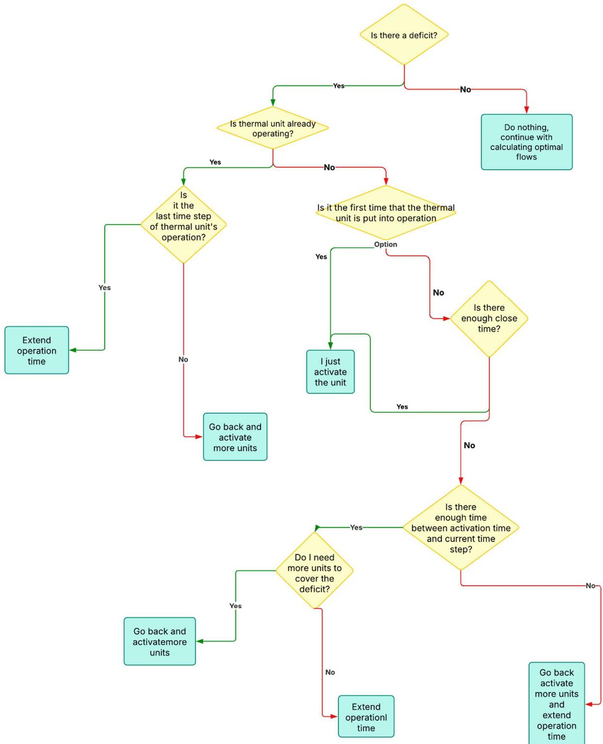
Figure 5.8 Flow Chart of thermal unit operation decisions
