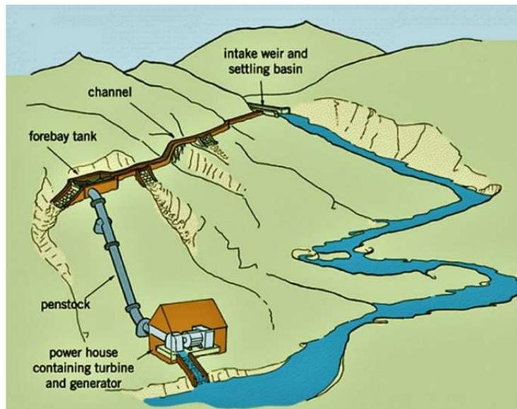
Figure 2.6 Typical layout of a run-off river plant (A. Efstratiadis, G.-K. Sakki & A. Zisos, *Small hydropower plants*)
