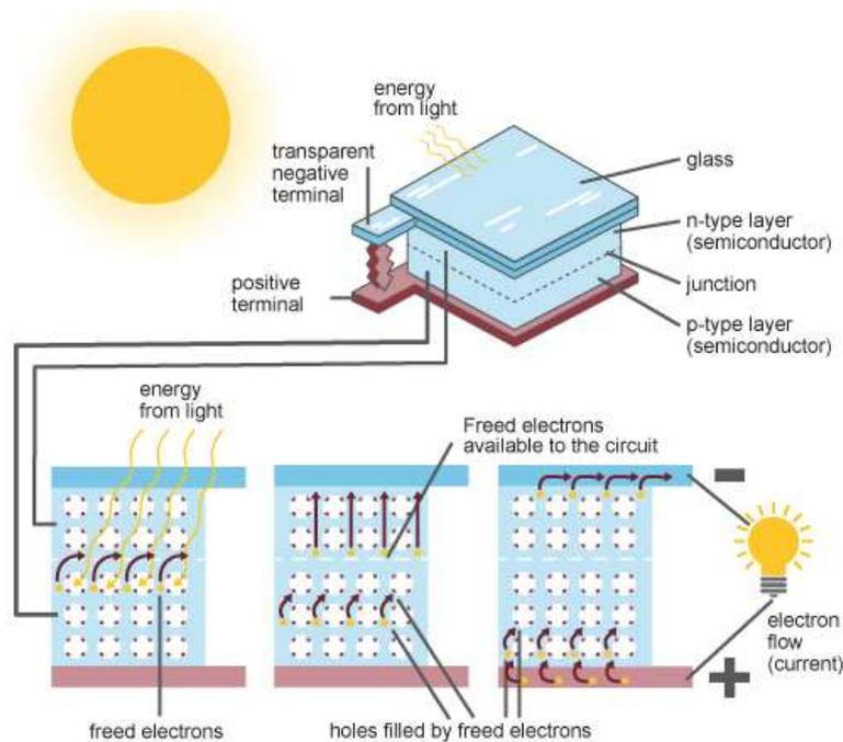
Figure 2.5 Inside a photovoltaic cell (U.S Energy Administration)
