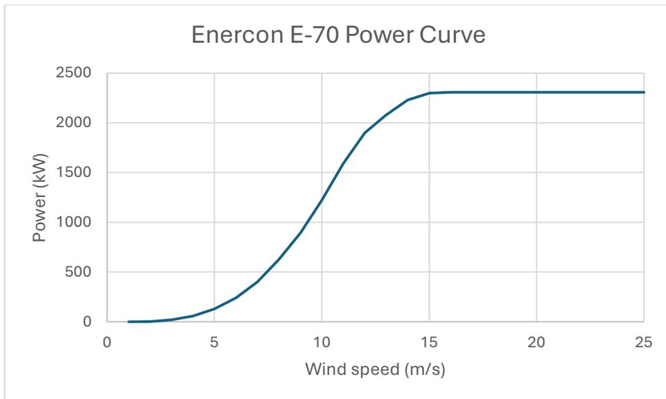
Figure 7.2 Enercon E-70 power curve
