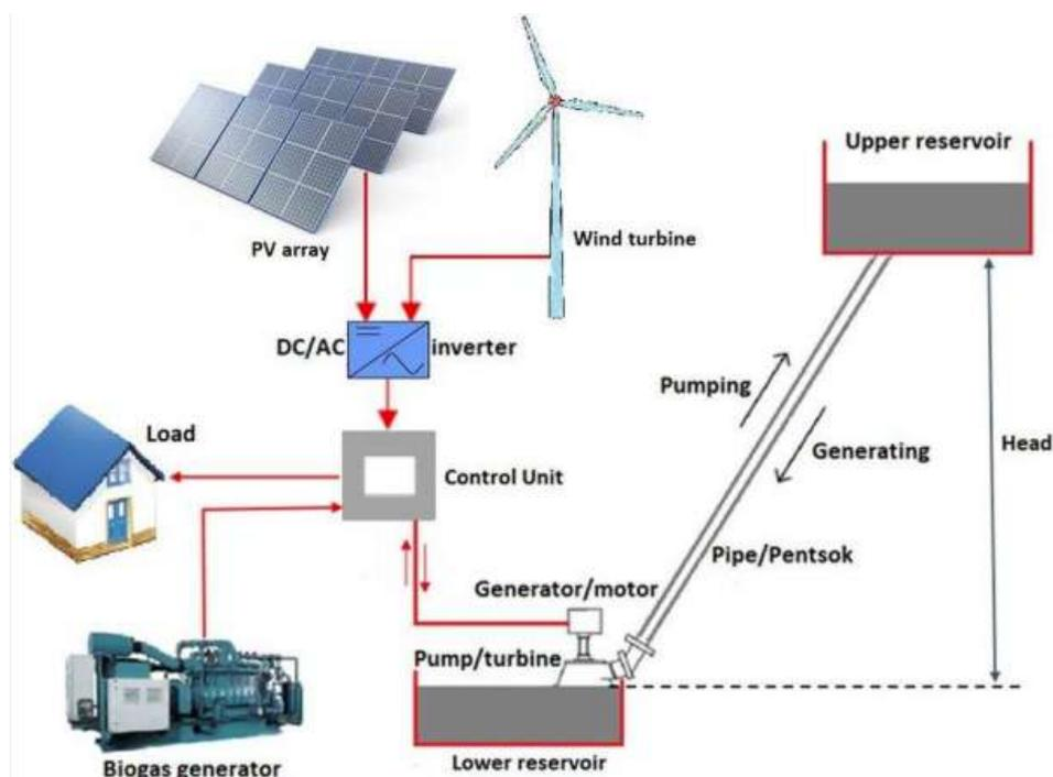
Figure 2.7 Typical layout of an HRES
