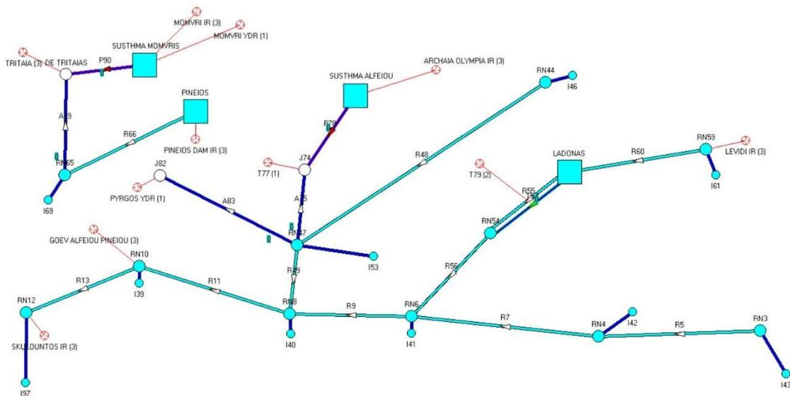
Figure 4.1 Example of network type schematization of Alfeios hydrosystem within Hydroneas (Kolioukou et al., 2024)
