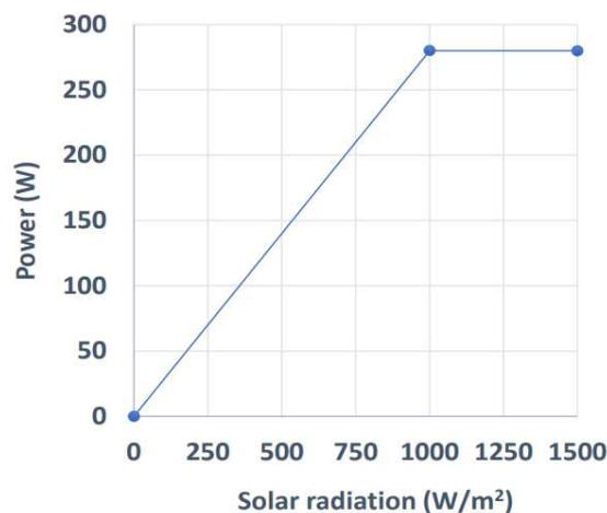
Figure 5.1 A typical power – solar radiation curve of PV panels (Efstratiadis et al., 2024)
