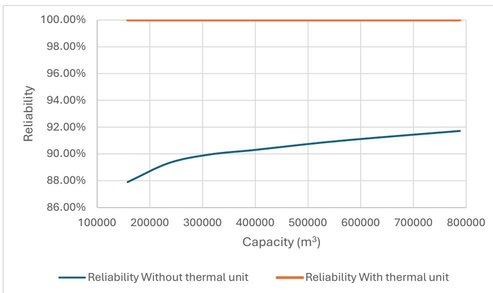
Figure 8.12 Reliability - capacity relationship with and without thermal units
