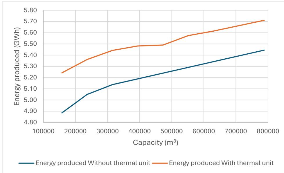
Figure 8.13 Energy produced - capacity relationship with and without thermal units
