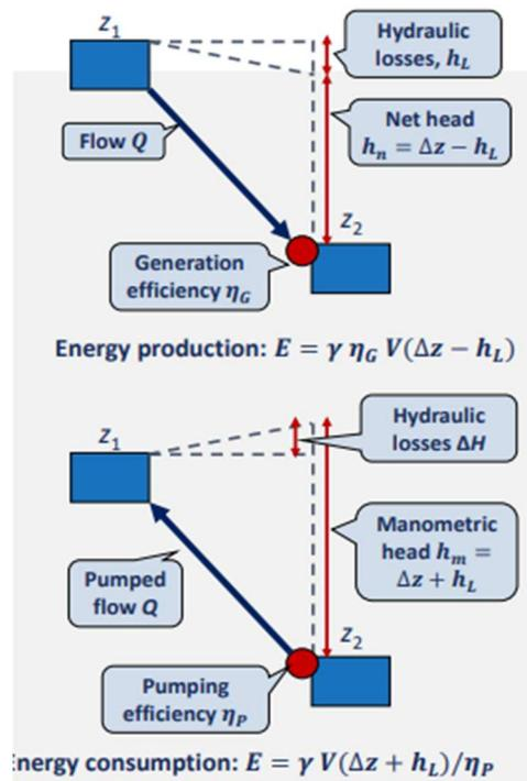
Figure 5.3 PHS system's energy consumption and production (Efstratiadis et al., 2024)
