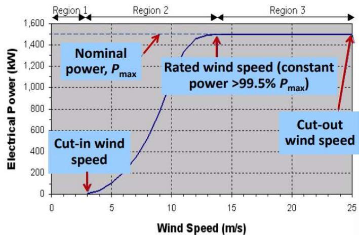
Figure 5.2 A typical power curve of wind turbines (Efstratiadis et al., 2024).
