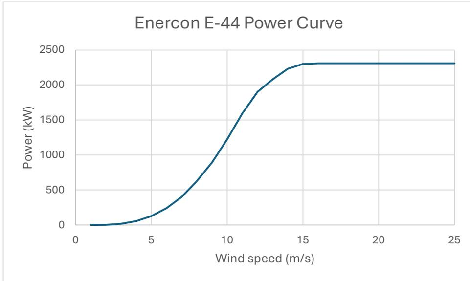
Figure 7.1 Enercon E-44 power curve
