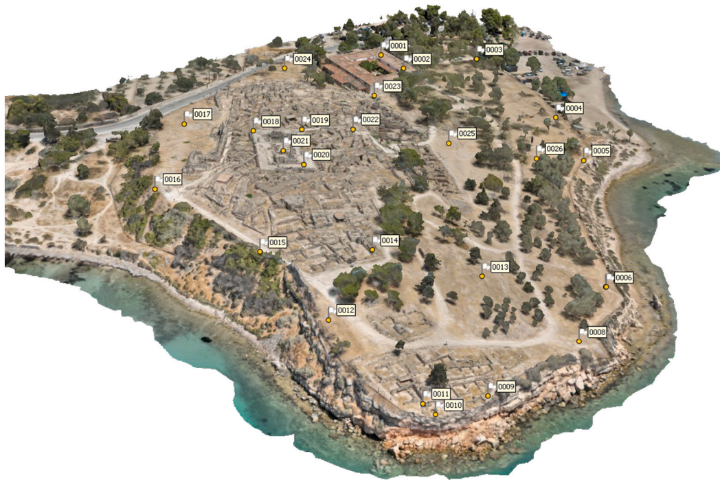
Fig. 5. Distribution of the GCPs measured in the archaeological site of the Temple of Apollo, superimposed on the textured 3D model of the site. CH angle from North to South.
