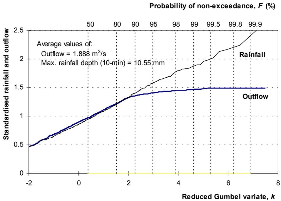
Figure 1. Conditional probability distribution functions of the maximum 10-minute rainfall depths ( $T = 5$  years) and peaks of outflow hydrographs at the outlet of the sewer system.
