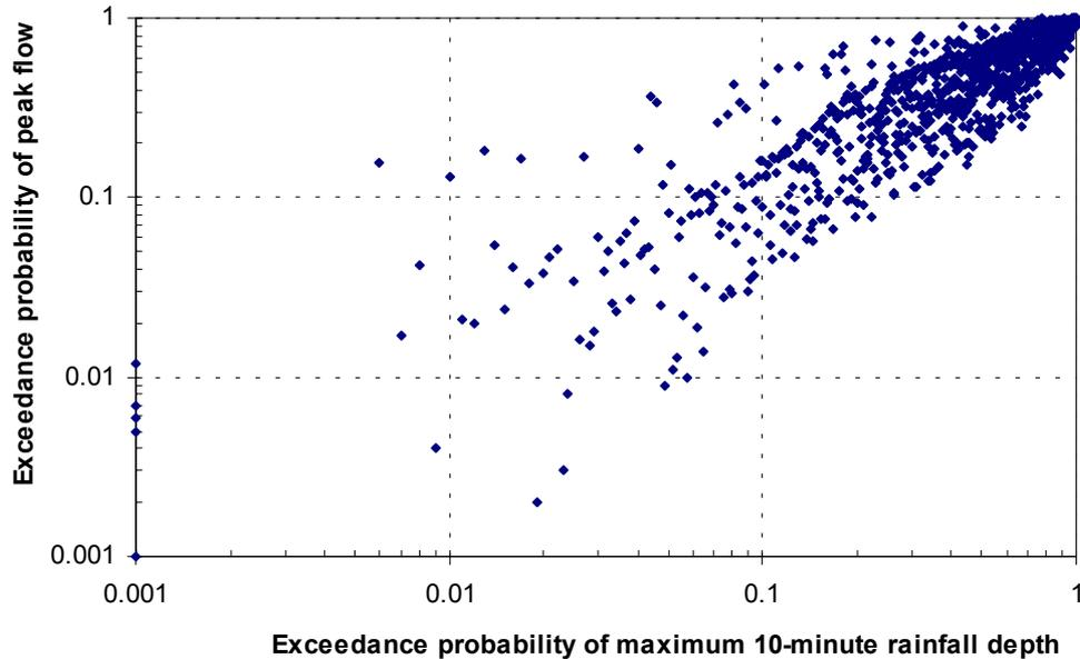
Figure 3. Plot of conditional exceedance probability of peak flow at the sewer outlet versus the conditional exceedance probability of maximum 10-minutes rainfall depth for the 1000 generated rainfall and flood events.
