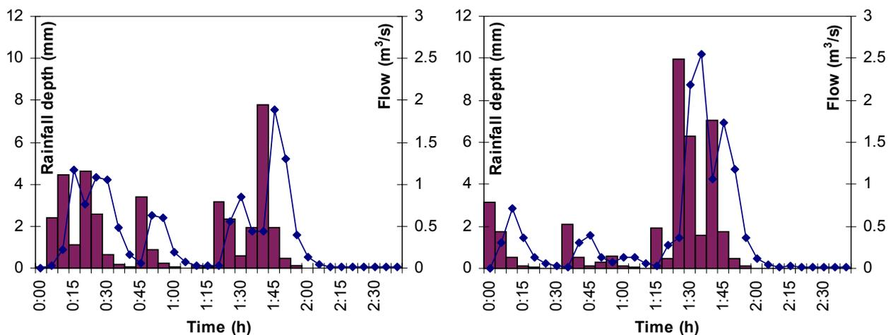
Figure 4 Examples of ‘design’ storms and floods generated by the proposed method: event corresponding to the average peak flow (left) and event corresponding to 90% non-exceedance probability for the peak flow (right).
