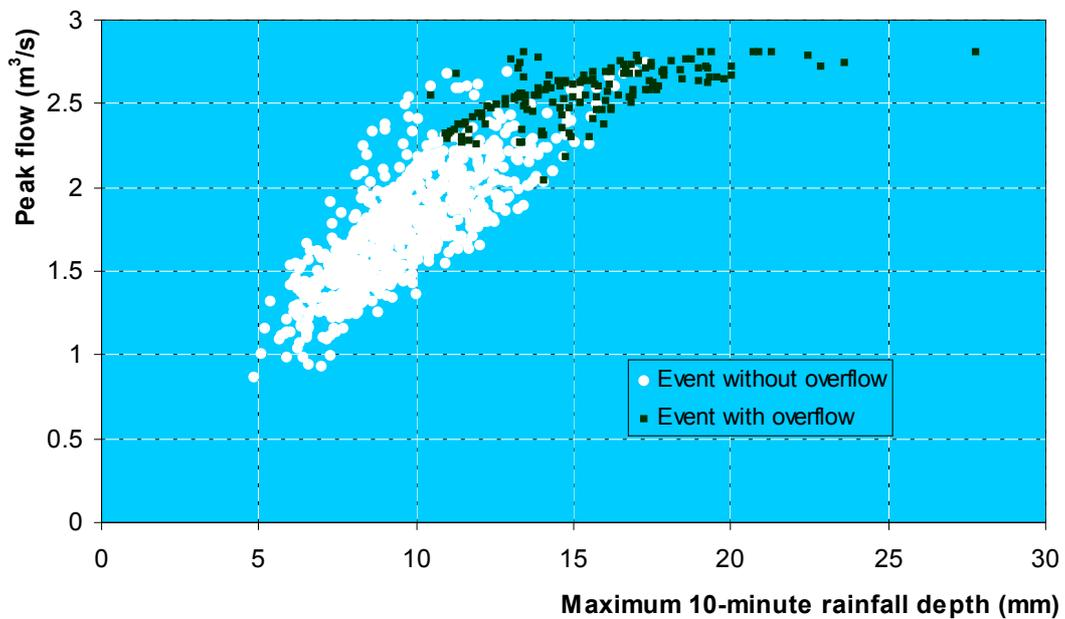
Figure 2. Plot of peak flow at the sewer outlet versus the maximum 10-minutes rainfall depth for the 1000 generated rainfall and flood events.
