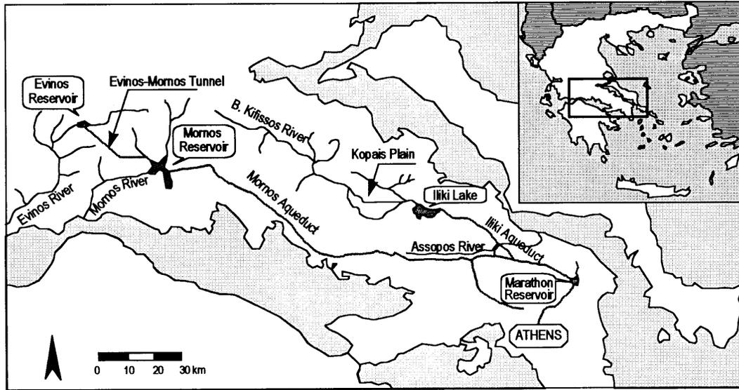
Figure 1. Layout of the Athens water supply system.
