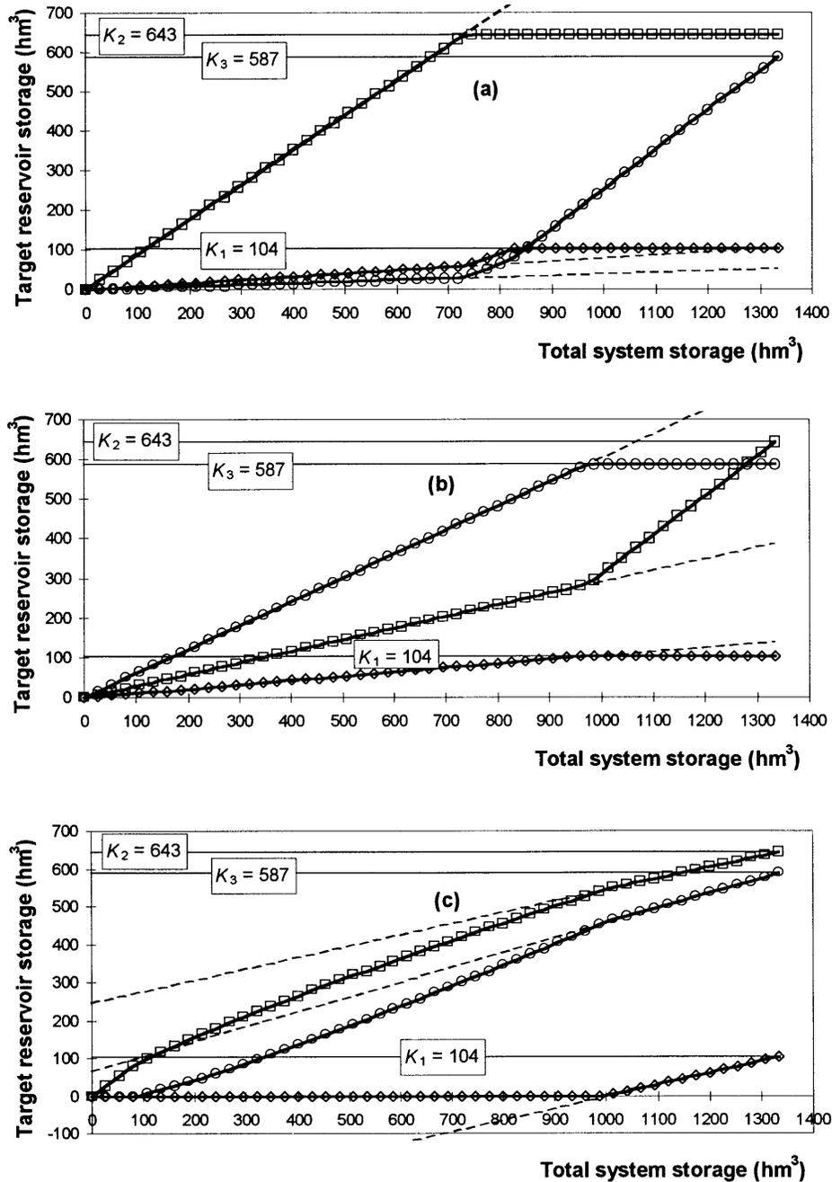
**Figure 6.** Graphical representation of operating rules for (a) the final parameter set of problem 1, (b) the final parameter set of problem 2, and (c) the parameter set of the space rule. Solid lines with rhombi, squares, and circles correspond to reservoirs 1, 2, and 3 (Evinos, Mornos, and Iliki), respectively, and represent the adjusted rule (equation (13)). Dashed lines represent the initial linear rule (equation (4)).
