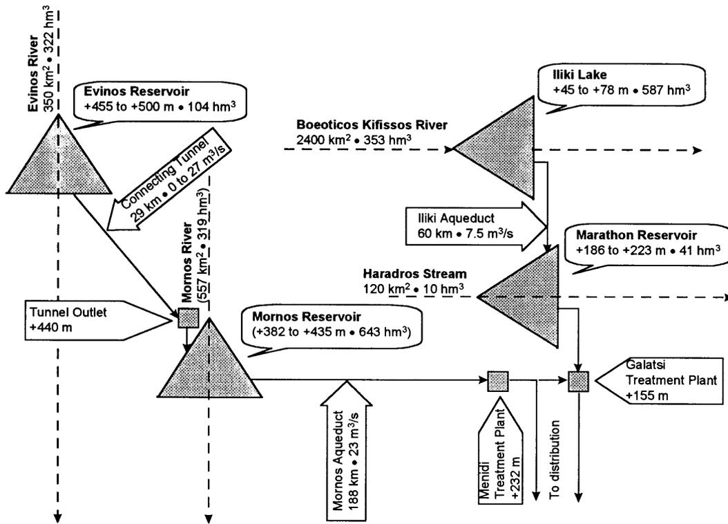
**Figure 2.** Schematic representation of the Athens water supply system. Characteristic data of the system are annotated: for rivers, the watershed area and the mean annual reservoir inflow; for reservoirs, the minimum and maximum water level and the active storage capacity; for aqueducts, the length and conveyance capacity; and for other components, the characteristic water levels.
