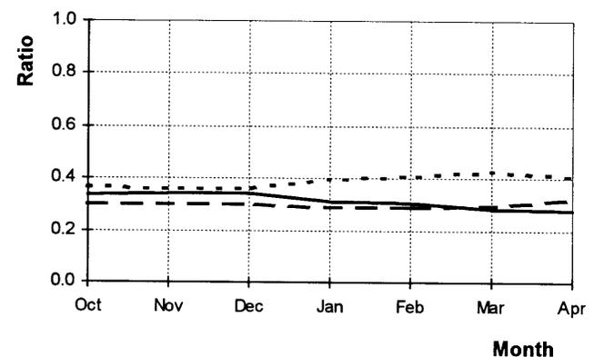
**Figure 5.** Ratios of cumulative monthly inflows into each one of the three reservoirs to the system cumulative monthly inflows ( $b_i$  in (8)). Cumulative inflows are considered up to the end of the refill cycle. Displayed values for the months of the refill cycle (October to April) are averages for the common period (for all reservoirs) of data availability (1979–1980 to 1987–1988). Continuous, dashed, and dotted lines correspond to the Evinos, Mornos, and Iliki reservoirs, respectively.
