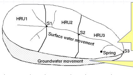
The catchment is divided into spatial subunits with similar morphological and hydrological characteristics (conceptual elements, not necessary sub-basins), called hydrologic response units (HRUs)
