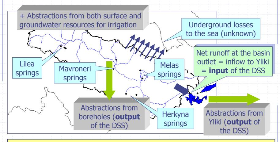
**Scope of the study**: Establishment of a simulation model to predict the actual inflow to Lake Yliki (compising of flood and spring runoff), for specific water supply and irrigation needs, fulfilled via both surface and groundwater resources
