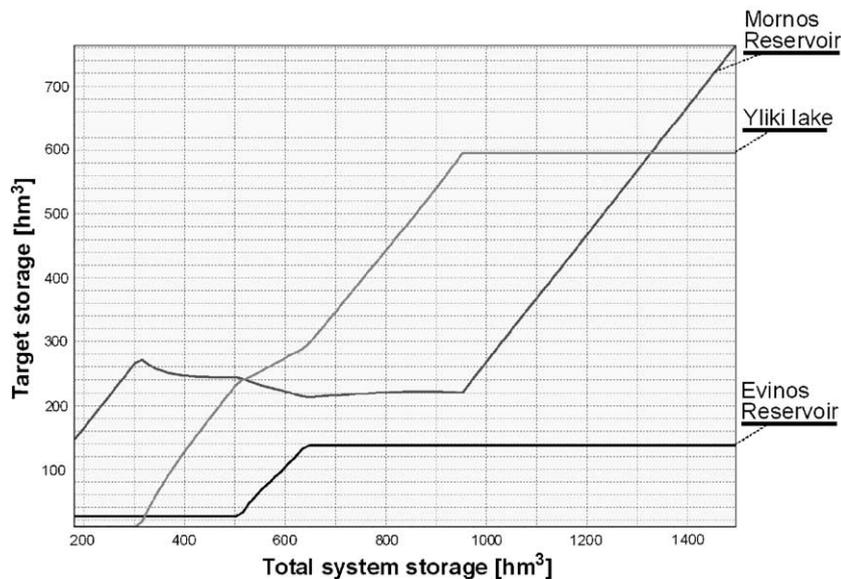
Fig. 6. Graphical representation of the optimal operation rules of the three main reservoirs of the Athens hydrosystem for Scenario 2.
