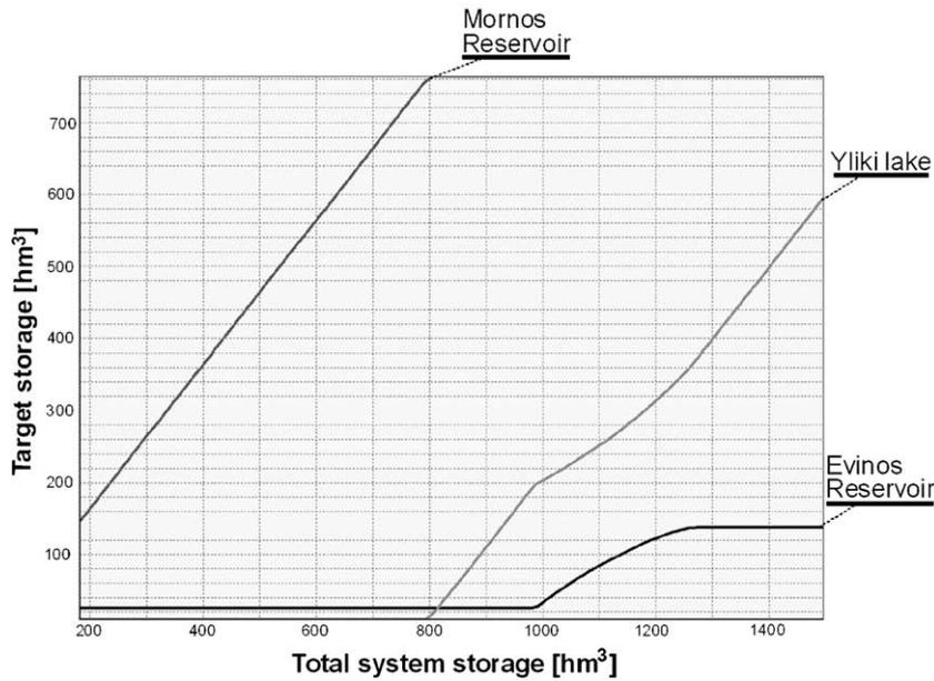
Fig. 5. Graphical representation of the optimal operation rules of the three main reservoirs of the Athens hydrosystem for Scenario 1.
