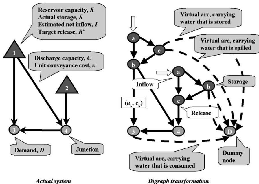
Fig. 3. An example of transforming a real hydrosystem into a digraph.
