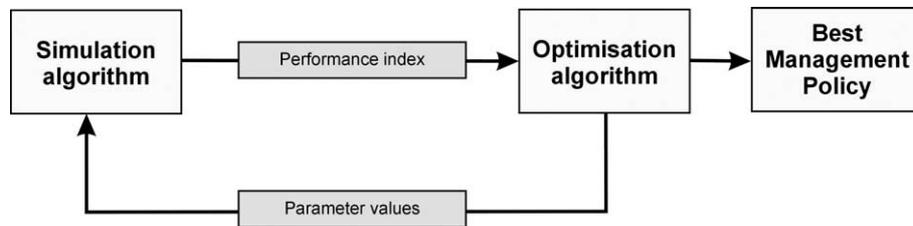
Fig. 4. Flow chart of the optimisation process.
