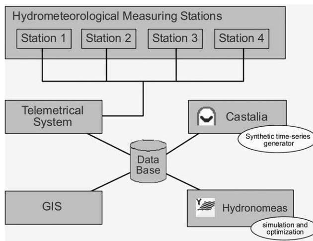
Fig. 2. The components of the DSS for the management of the Athens water resource system.
