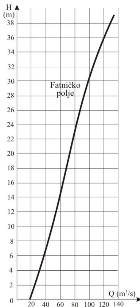
**Figure 17.** The estimated relationship of flood level (H) and the cumulative swallow capacity (Q) for Fatničko Polje
