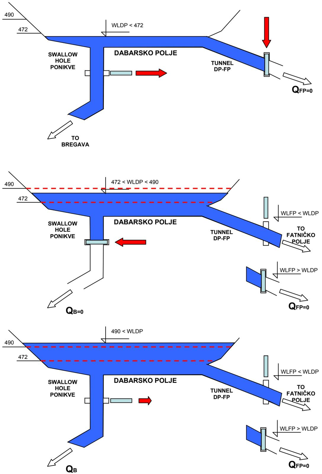
**Figure 10.** Conditions for flow regulation - operation of the tunnel
