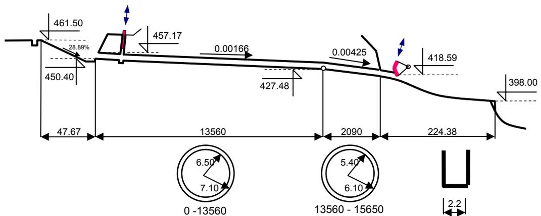
**Figure 8.** Longitudinal section of the tunnel between Fatničko polje and Beleća reservoir
