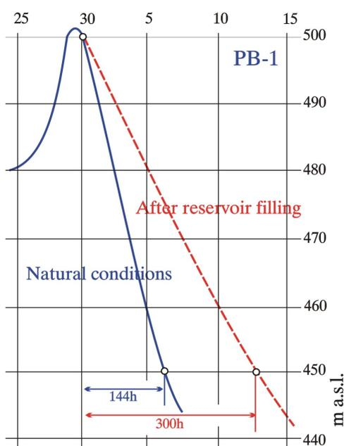
**Figure 19.** Water table recession curve in borehole PB-1
