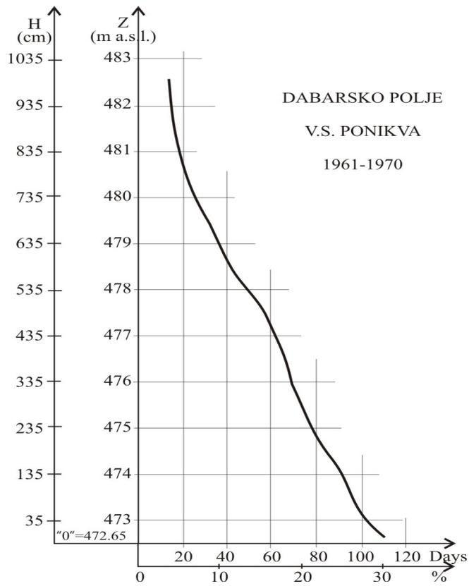
**Figure 23.** Duration diagram of annual flood in Dabar Polje in the zone of gauge station Ponikva, under natural conditions (Paviša, 1983)
