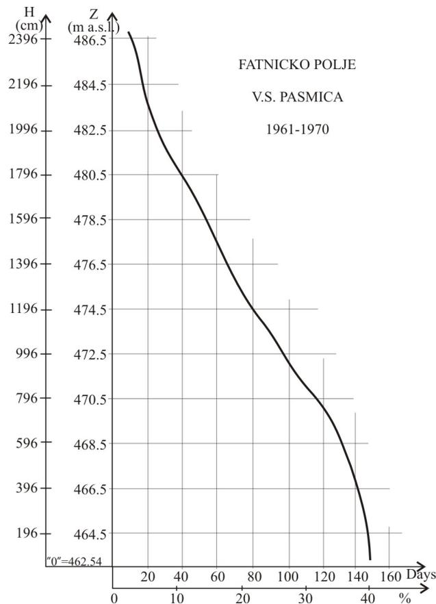
**Figure 18.** The annual flood duration curve of in Fatničko Polje under natural conditions in the zone of the Pasimca gauging station (Paviša, 1983)
