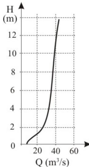
**Figure 22.** The relationship of flood level (H) and the cumulative swallow capacity (Q) for Dabarsko Polje
