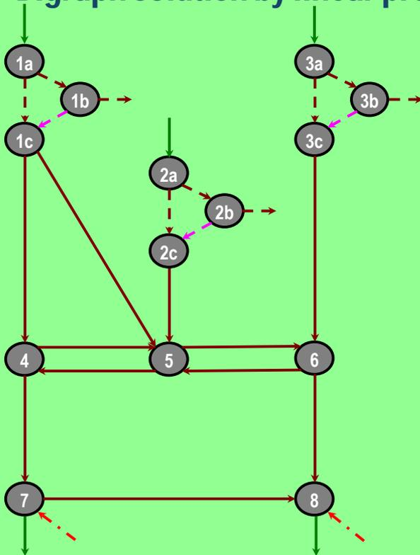
Determine all unknown discharges  $Q_{ij}$  at edges  $ij$ , by **minimizing total cost**
