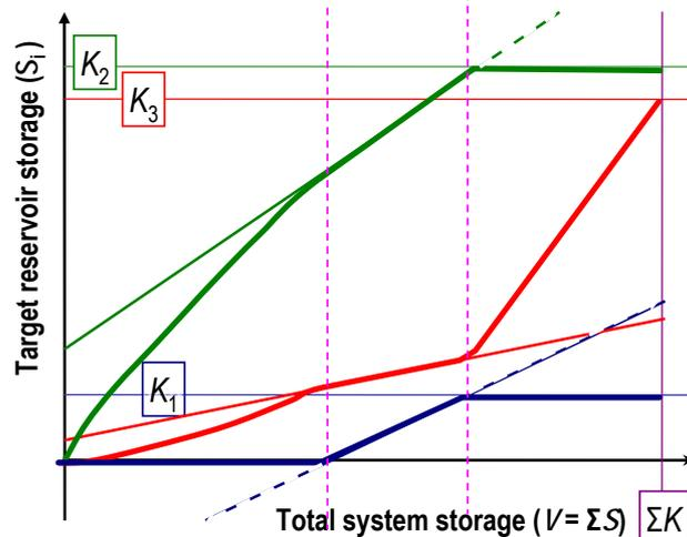
**Two parameters** per reservoir ( $a_i, b_i$ ) = **Control variables**
