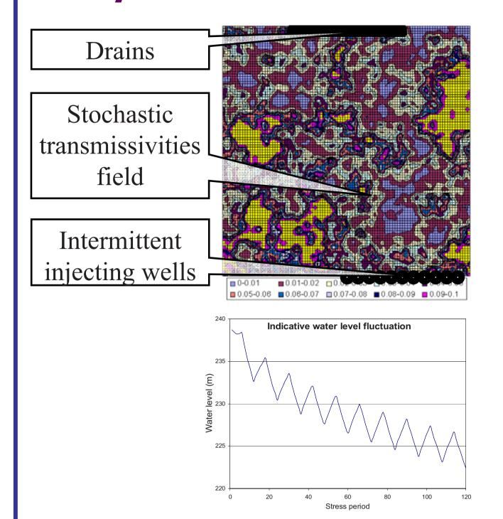
A 2D stochastic model is used to produce 100×100 synthetic transmissivity values (Theodoratos, 2004).
