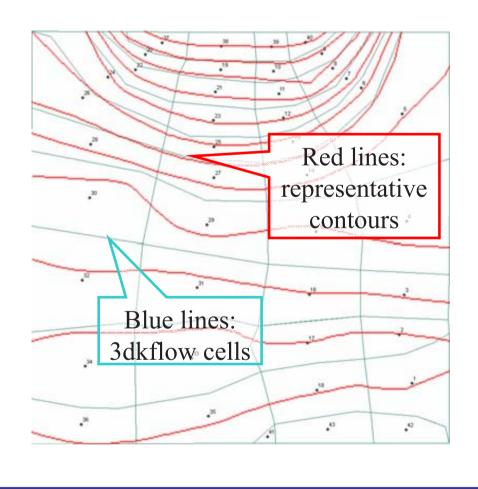
The concept of the 3dkflow model is described by Rozos and Koutsoyiannis (2005) and by Rozos and Koutsoyiannis (2006). The 3dkflow cells design was based on the most representative contours map for the whole simulation of the hypothetic aquifer.
