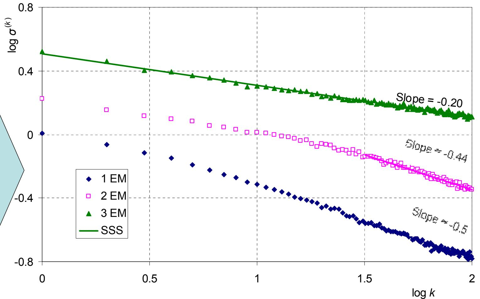
The slope of the logarithmic plot (as  $k \rightarrow \infty$ ) is  $H - 1$  where  $H$  is the Hurst exponent. The slope in the “1 EM” case is  $-0.5$ , i.e.  $H = 0.5$ , meaning no Hurst-Kolmogorov behaviour.
