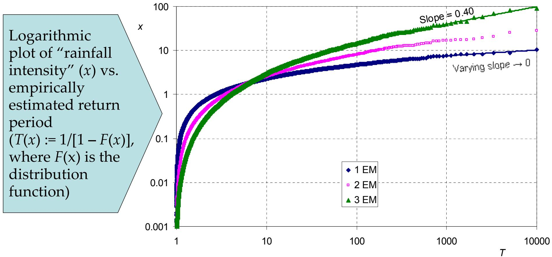
As the number of processes in the chain increases, the right tail of the distribution moves toward higher “rainfall intensity” values and its shape changes from exponential type to power type; simultaneously the probability density becomes infinite for  $x = 0$ .
