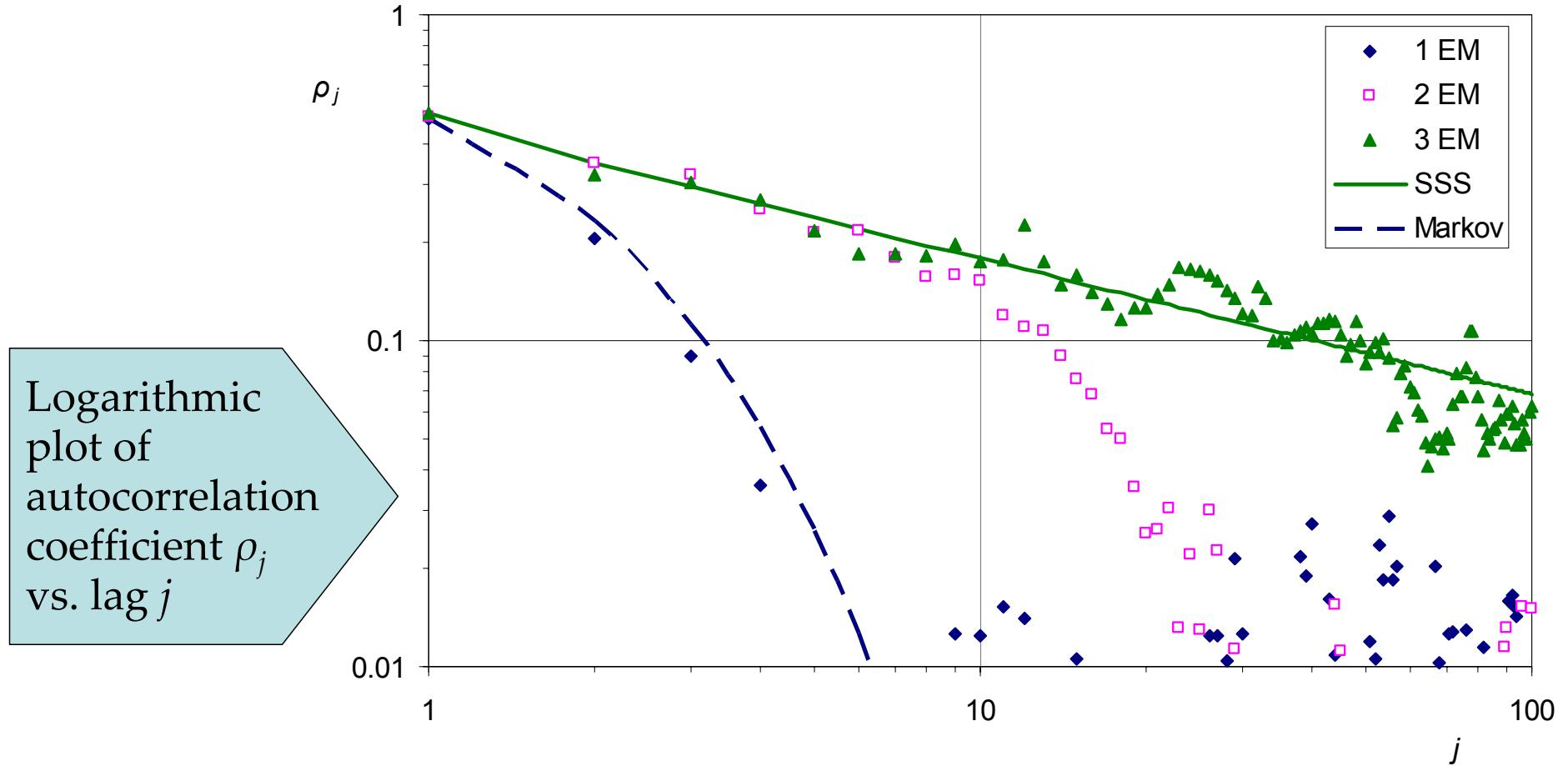
As the number of processes in the chain increases, the shape of the autocorrelation function changes from Markovian (exponential decay – short range dependence) to power type (long range dependence).
