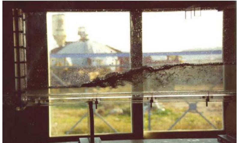
Figure 9. Development of turbulence in a hydraulic jump in a controlled experiment in laboratory, whose window, with the help of reader's imagination, reveals the outer uncontrolled turbulence (courtesy of Panos Papanicolaou).
